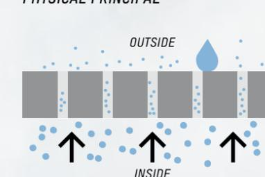
Water droplets Water vapour molecules Hydrophilic polyether Hydrophobic polyester
